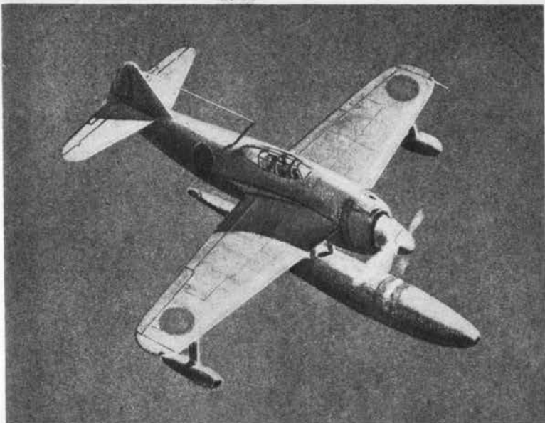
REX The seaplane fighter from which George ( opposite ) was adapted, Rex is probably replacing Rufe. Except for single float, larger spinner and more pointed tail, Rex closely resembles George.
